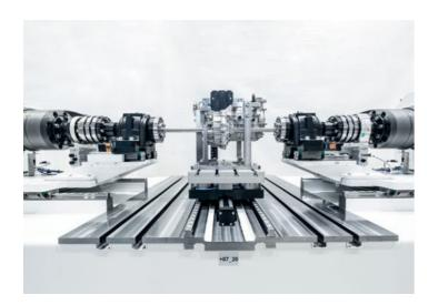
E-Drive test bench for electric axle drives
