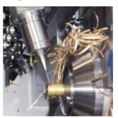
Tool measurement – TC76 with protective sleeve
